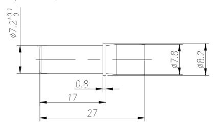
Adaptationrange of crimping wire: 6awg  $^{\sim}$  8awg (13.3mm)  $^{2}\sim$  8.367mm  $^{2}$ ).
