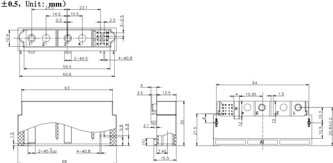
Note: 1) the power pins shall be installed in holes 1 and 3, and the signal pins shall be installed in holes 5, 6, 11 and 12;
