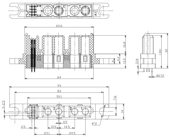
Note: the power jacks shall be installed in holes 1 and 3, and the signal jacks shall be fully installed and connected;
